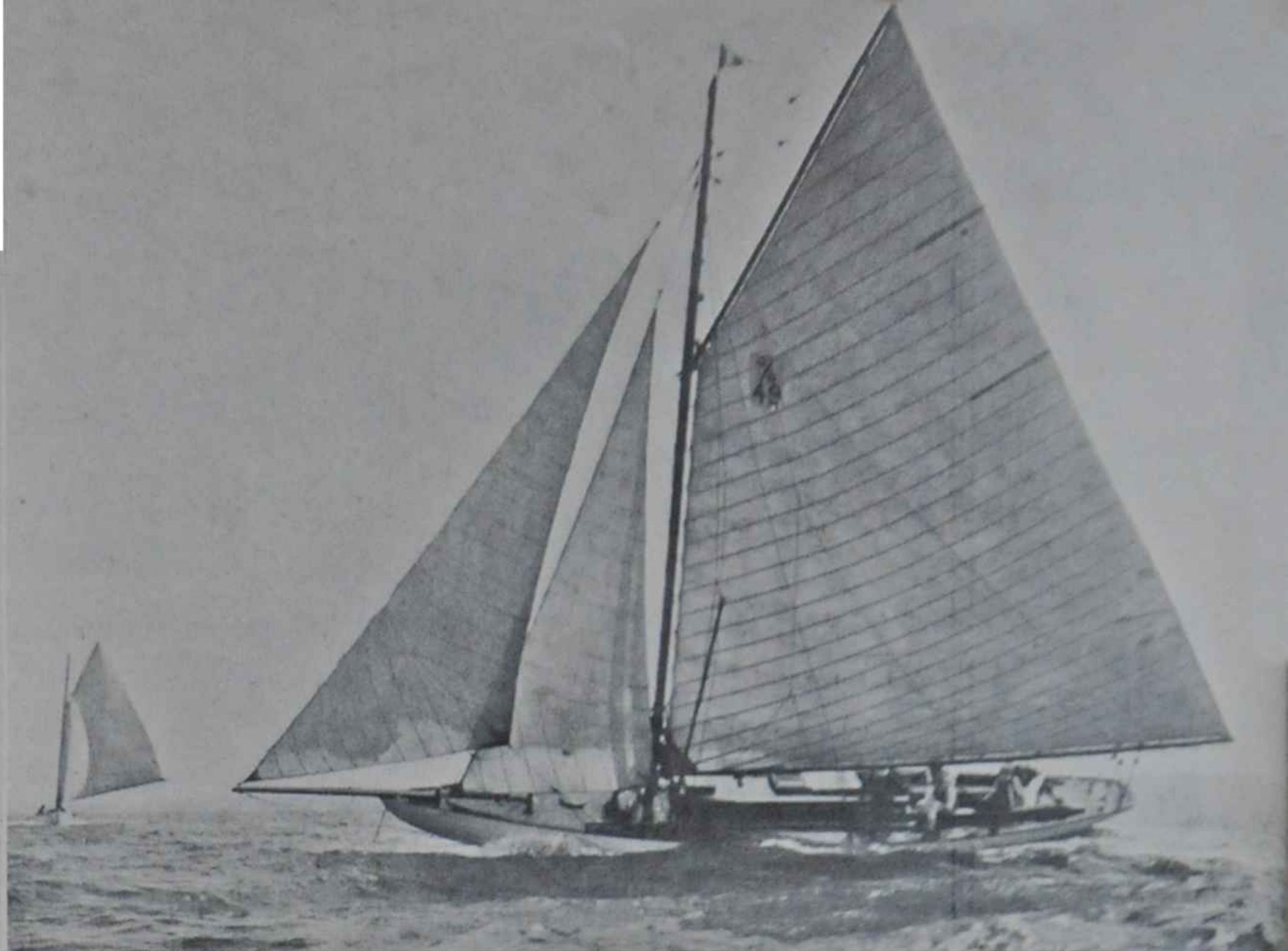
Above, "Mashnee" as she came from the Herreshoff shop in 1902. Her big rig made her a handful in a breeze. Left, the intermediate rig, with single headsail, improved her efficiency and simplified handling
