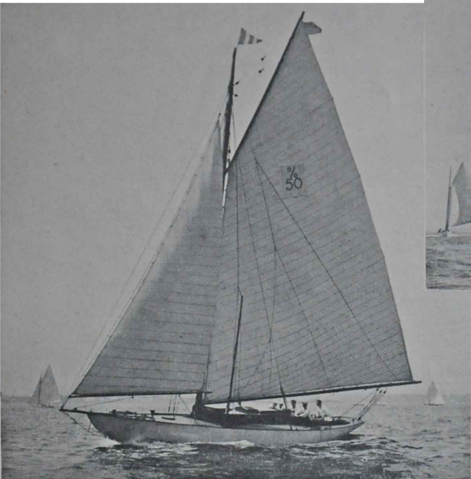
Above, "Mashnee" as she came from the Herreshoff shop in 1902. Her big rig made her a handful in a breeze. Left, the intermediate rig, with single headsail, improved her efficiency and simplified handling
