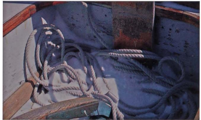
**7. Randomly stowed lines like these will not develop the mildew problems that invariably beset tightly coiled cordage, and the light layer of snow here will protect the wood from sun damage, salt spray and rain.** Notice how any fastening problems in the cockpit or the lazarette hatch can be spotted quickly where bungs have been allowed to pop out. A simple scrape-and-paint procedure will do come spring. The paint drip on the tiller jaw should be removed.
