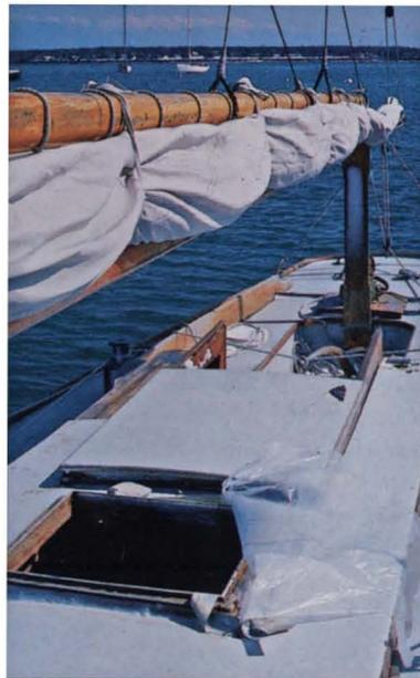
**2. A boat should always be left as open as possible during extended periods of non-use.** Sails bent on, lines a-ready, this Herreshoff classic is just about set to go come spring. Note the use of duct tape and small pieces of polyethylene as coverings for small openings. These materials "give" under extreme conditions, rather than creating tiny pockets of resistance that can place undue local stresses on the boat.
