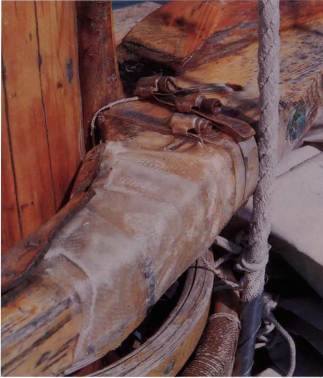
**4. The march of progress in materials technology is clearly evident in this photograph.** When *Beaux Eaux* was launched in 1904, chafe was handled by leather pads, canvas and servings of small stuff. Bolts, nails and rivets were the only fastenings; all put great strains on small areas. Eighty years later we have corrosion-proof variable-stress metal strappings and wraps of fiberglass to distribute loads evenly. Easy-to-apply tapes deal with chafing.
