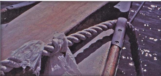
**5. Simple materials are the best.** Too many “sophisticated” boat owners would frown on this use of shredded trash bags as an anti-chafe measure, yet this material is unaffected by the elements, holds its color even after constant exposure to bright sunlight and has a frictional coefficient very close to zero. The same can hardly be said for marline serving or those heavy rubber-and-leather devices sold as “chafing gear.”
