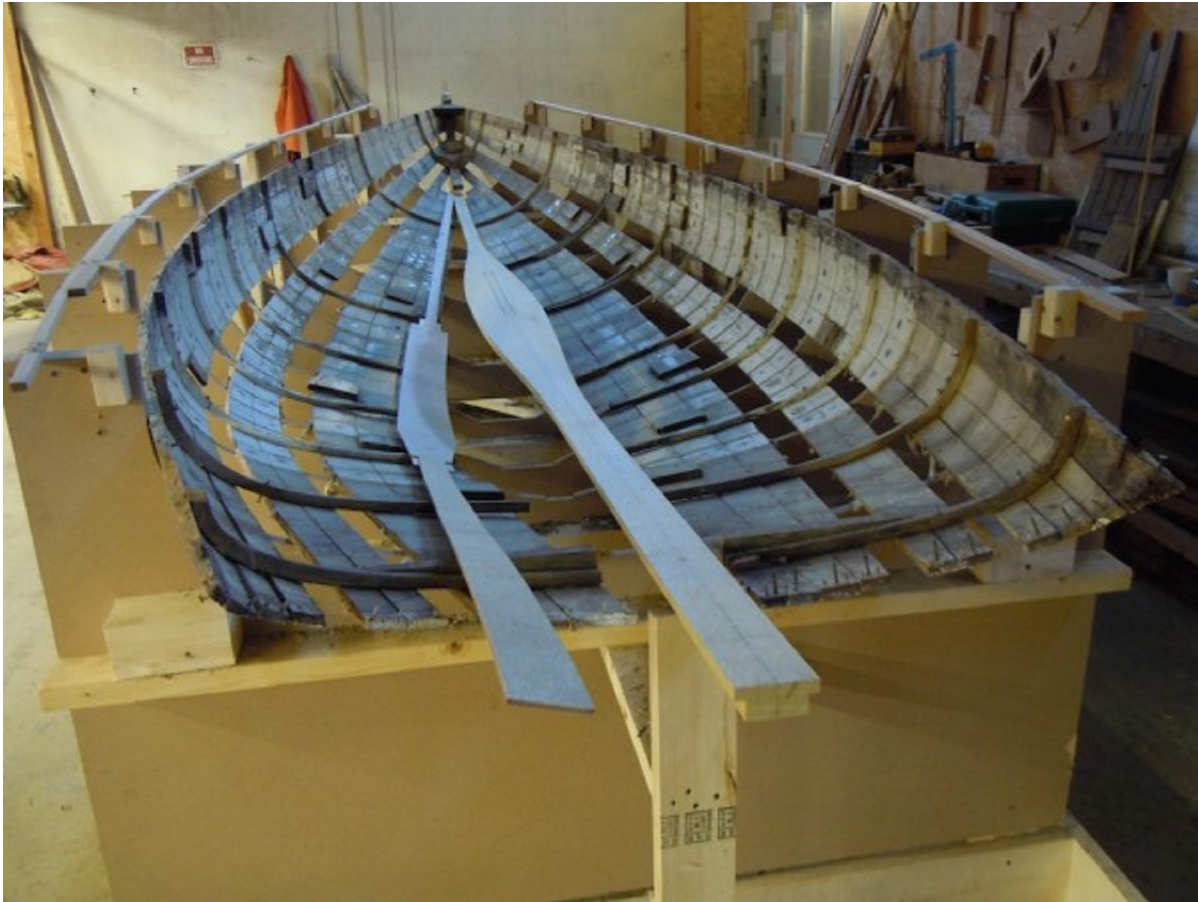
A new keel timber of iroko, built to the pattern lying next to it, is about to be steam-bent into place under the hull.
