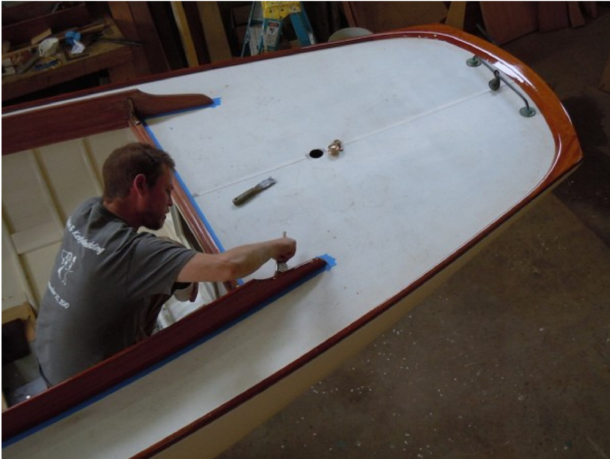
Trim done, now it's varnishing time.
