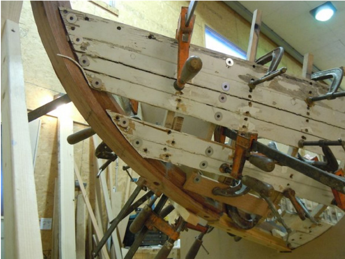
Here is the stem whose shape came directly from the designer's dimensions.
