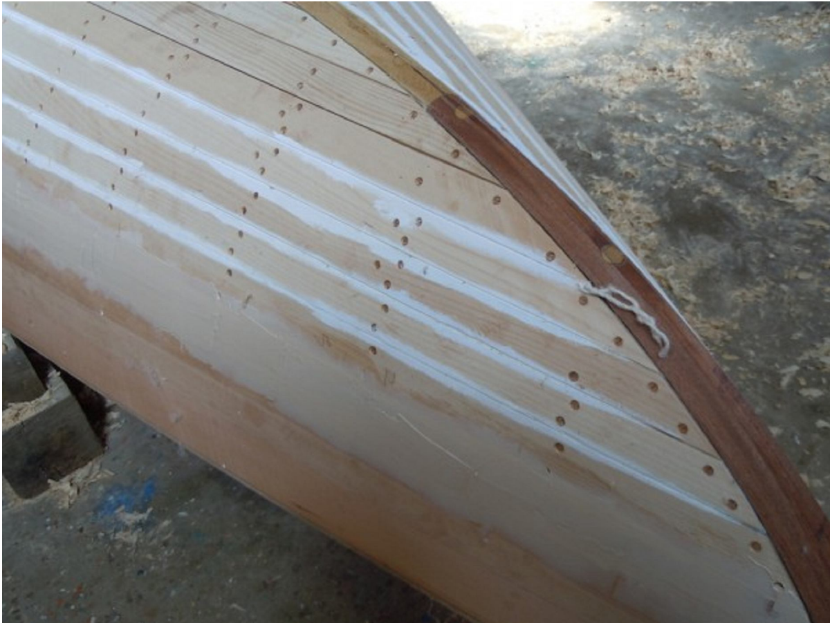
After planking, fairing, and caulking, KRISTIN is about ready to be turned back rightist-up.
