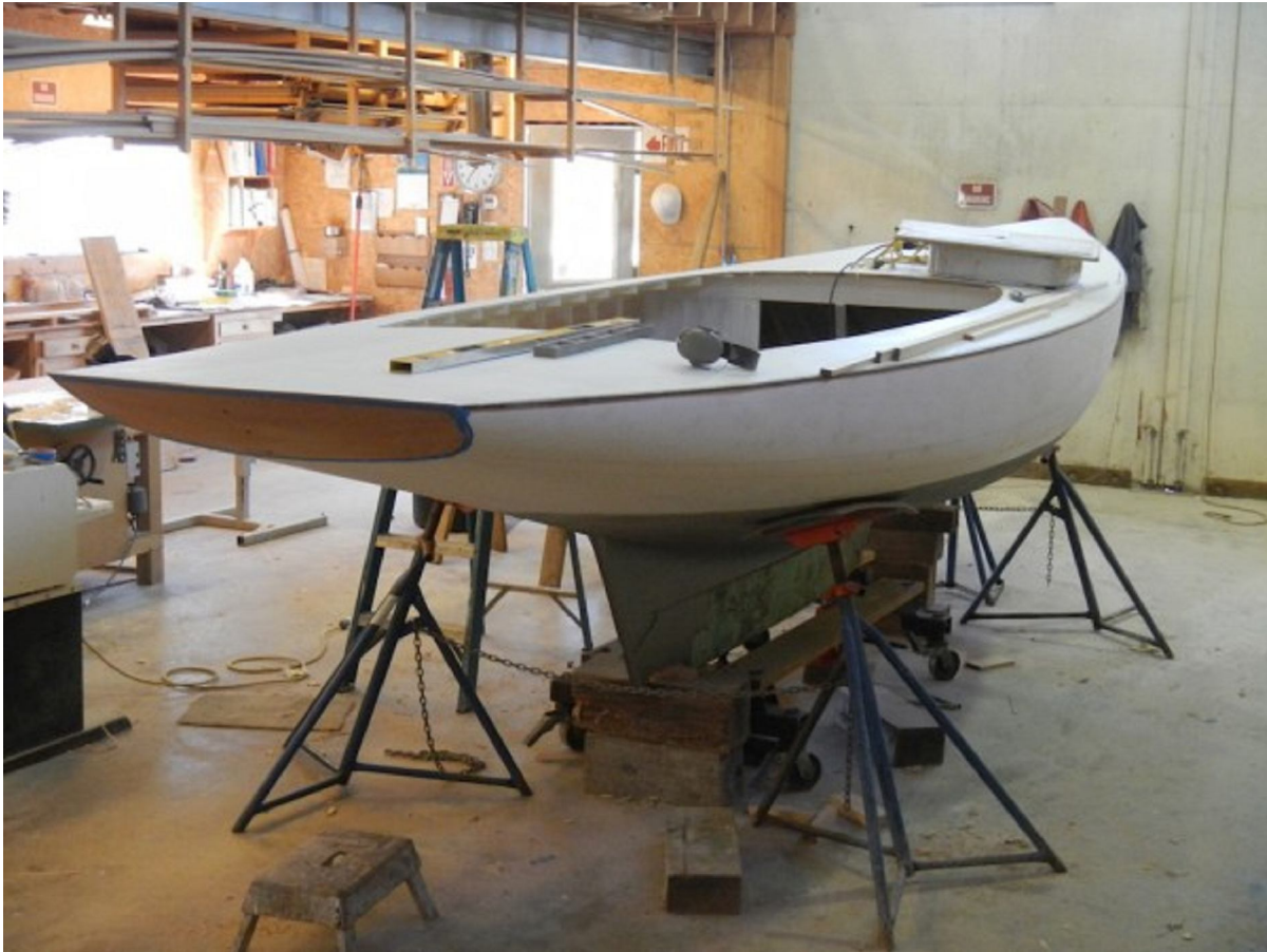
All decked, this time with Dynel-sheathed plywood, she's ready for floorboards and trim,
