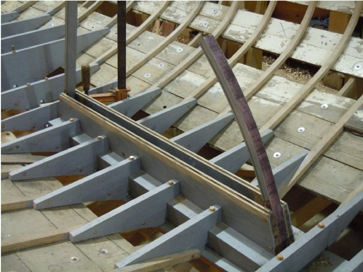
Bedlogs and end posts for the centerboard trunk.
