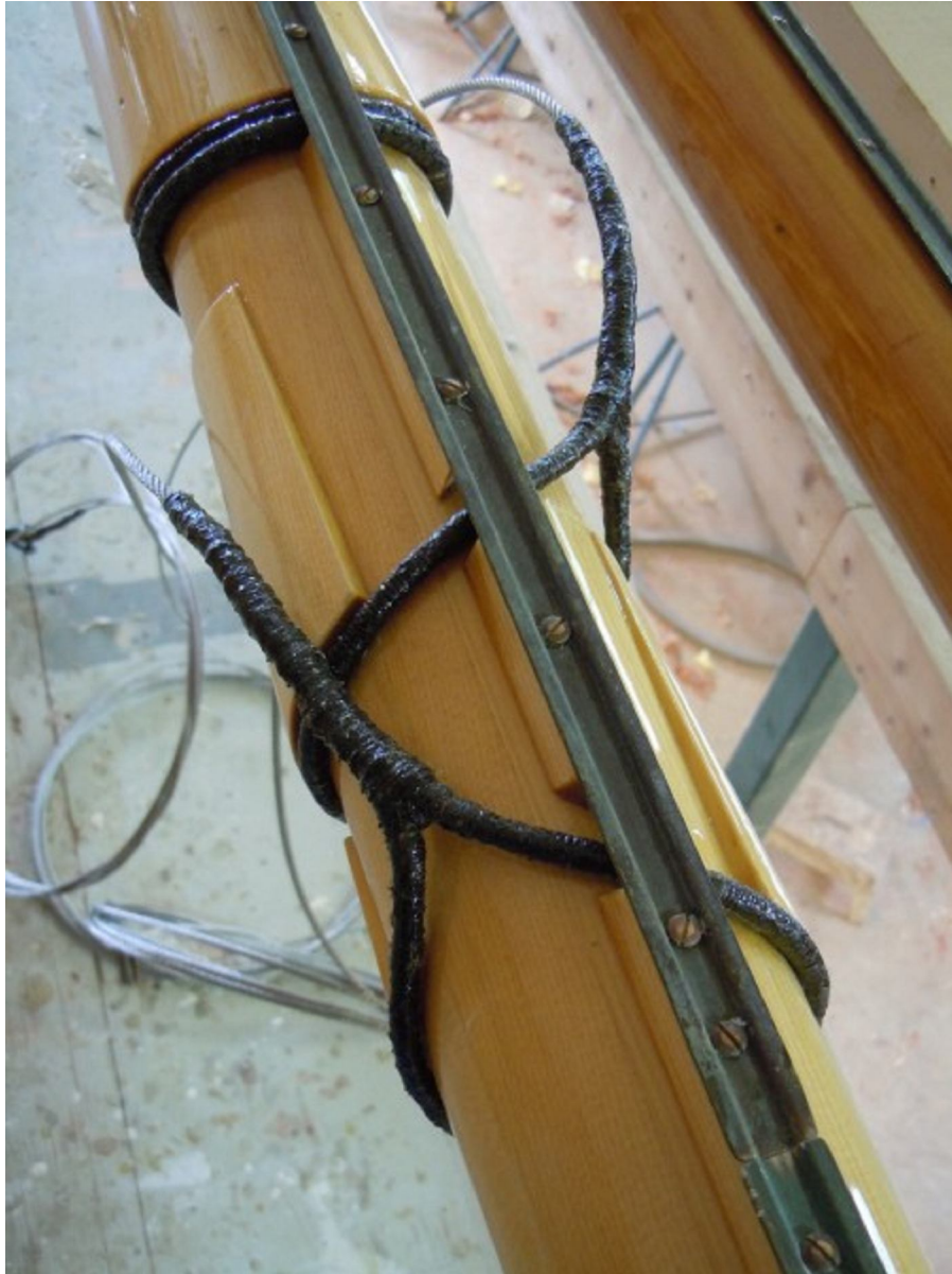
A new hollow mast with spliced rigging, just like when new.
