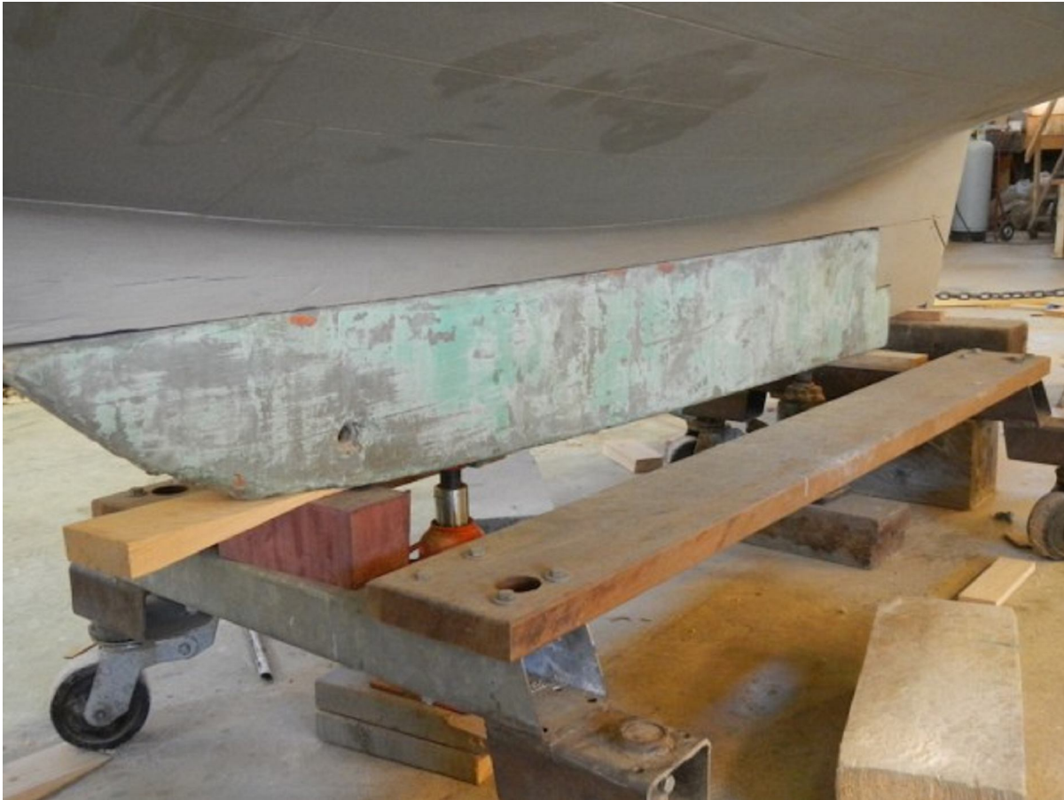
Ballast keel being jacked into position.
