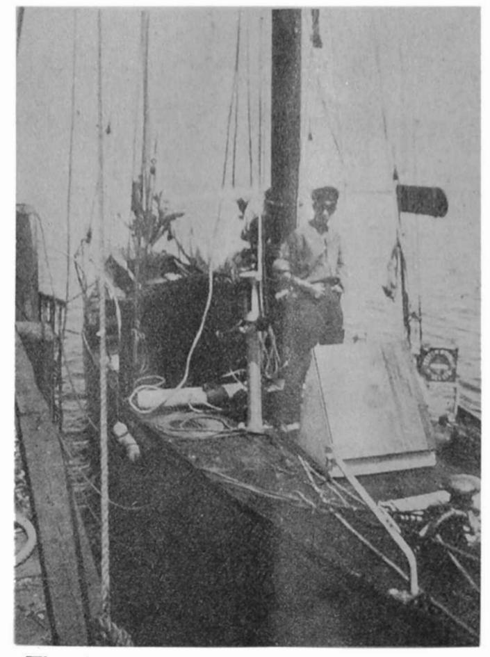
The forward deck, showing hood for forward hatch to keep out water
