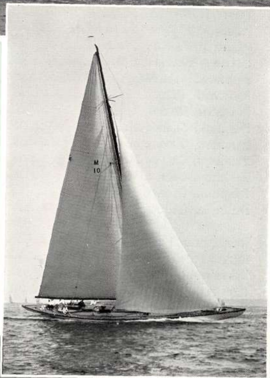
"Istalena." Oak framed double planked "M" Class sloop. Designed by Mr. L. Francis Herreshoff of Marblehead and built by Herreshoff Manufacturing Company. Proved to be one of the fastest of her class, with ample cruising accommodations.
