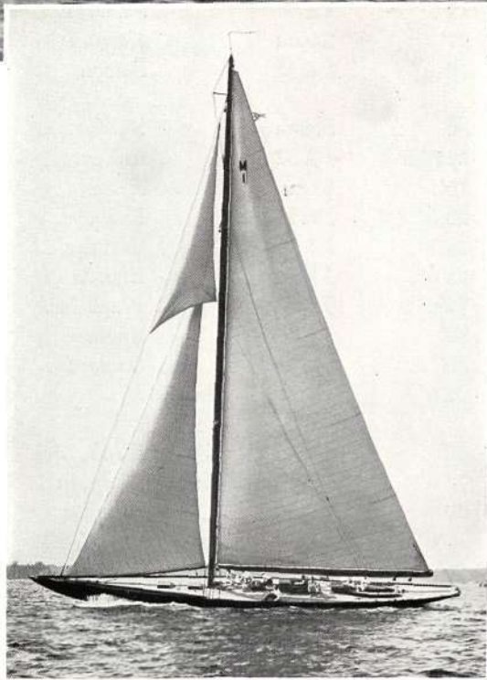
"Prestige." Steel framed mahogany planked "M" Class sloop. Designed by Burgess & Morgan, built by Herreshoff Manufacturing Company. Has an enviable record.
