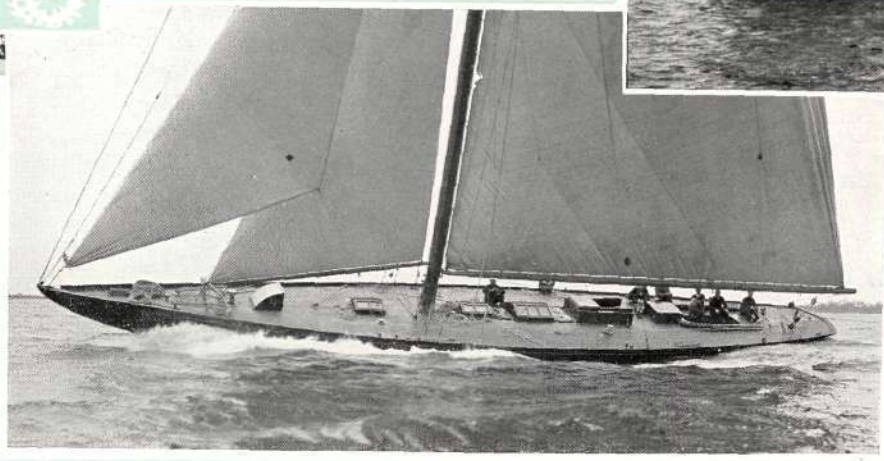
"Sheerness." Steel framed mahogany planked "L" Class sloop. Designed and built by Herreshoff Manufacturing Company. Combines unusually good speed with a beautifully appointed interior.
