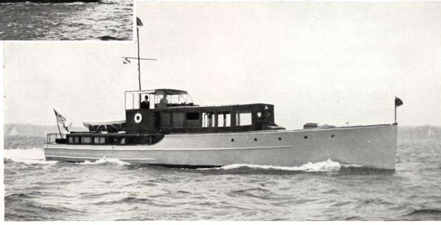
"Shuttle." Seventy foot high speed commuting boat. Oak framed and double planking. Unusually able and sea-worthy hull, with a maximum speed of twenty-seven miles per hour. Designed and built by Herreshoff Manufacturing Company.
