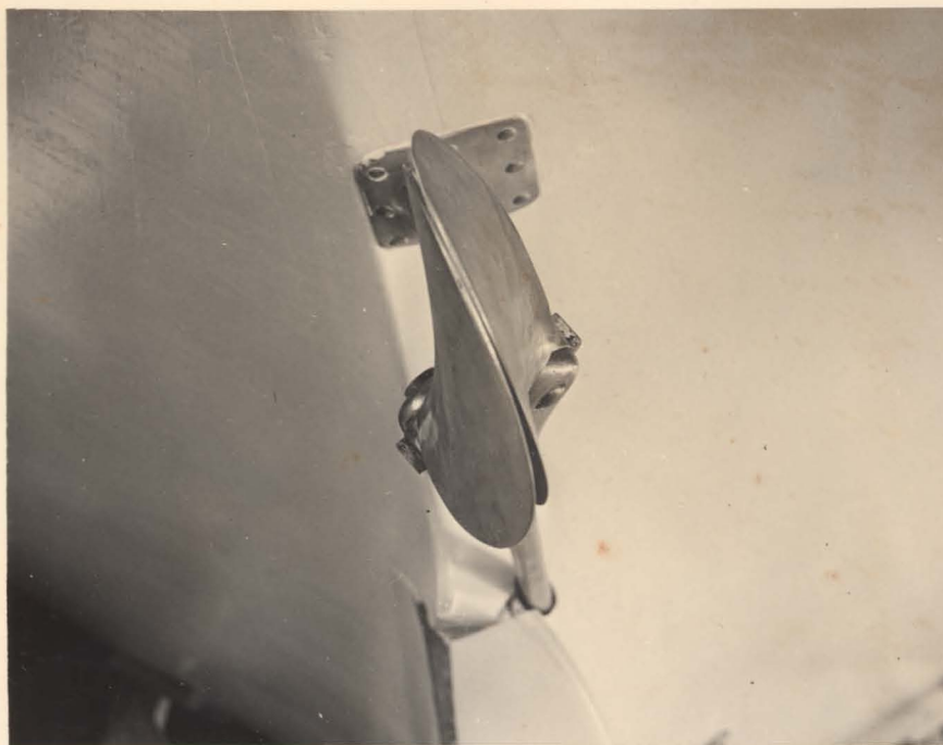
THE HERRESHOFF FOLDING PROPELLER (In closed position)
