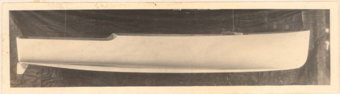
A "towing model" developed for experiments in the U.S. Navy tank at Washington.
