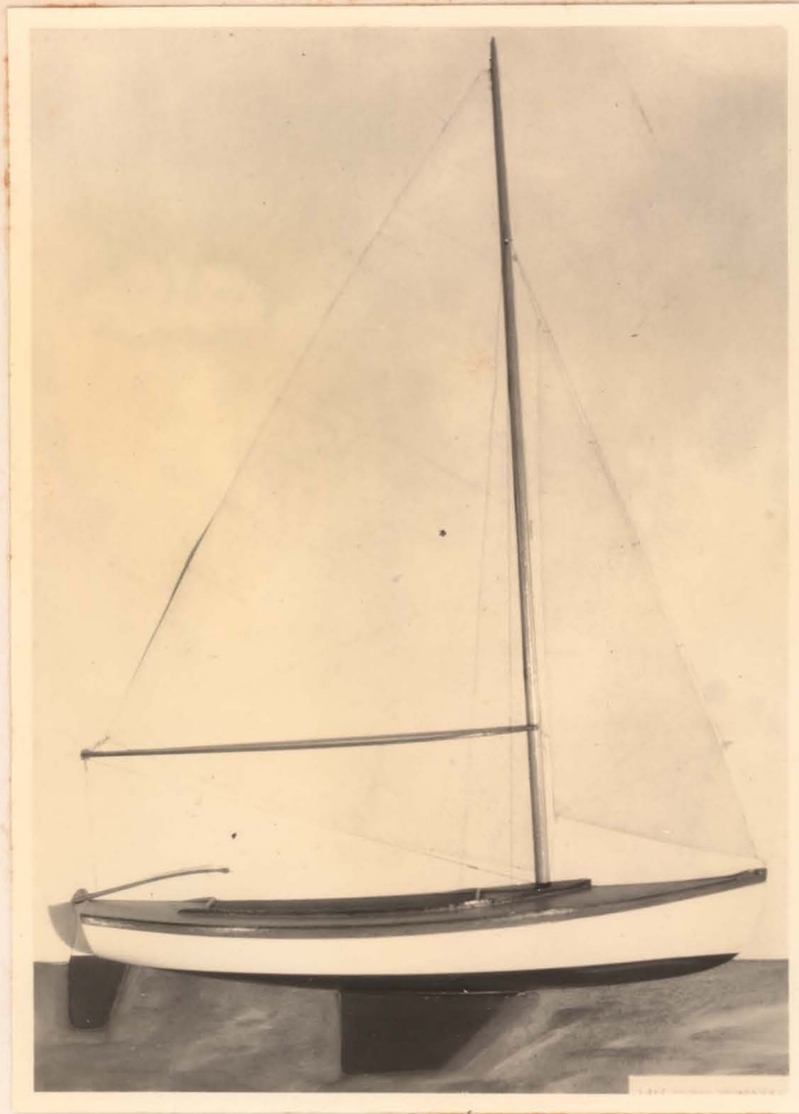
A half-model including spars, deck-erections, rigging and canvas sails.
